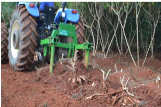
*Efficient TEK Mechanical Cassava Harvester in operation*
